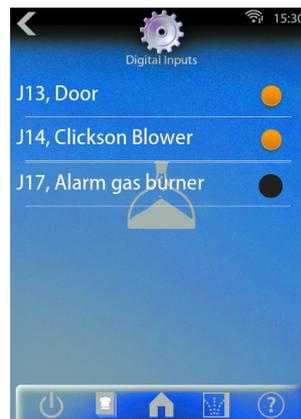
"Digital inputs" is showing the available inputs and also which contacts are closed.
