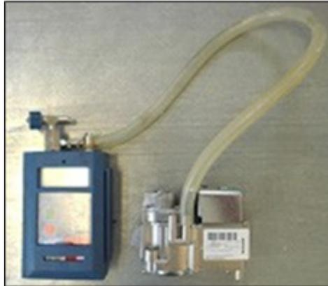
Gas inlet: Inlet of gas after gas pressure reduction valve (max. 22" H<sub>2</sub>O).
