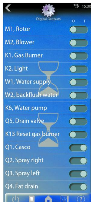
"Digital outputs" is showing the available outputs and also which are activated.
