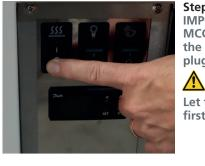
Step 1 IMPORTANT: turn off the MCC by pressing the O on the 3 switches. Pull the plug.
