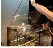
Step 4 Lift and hold the top glass pane while removing the transparent air guide pane for cleaning.
