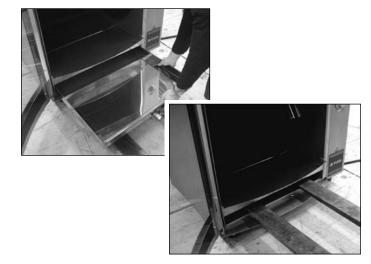
Another possibility is to disassemble the pallet. For the pallet of the STG 7 and STW 7 follow the procedure on the photo.
