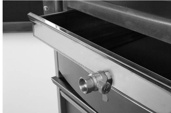
Drain valve closed. (Handle vertically)
