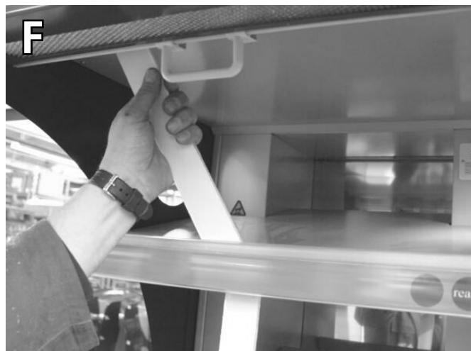
Remove top transport safety beam
