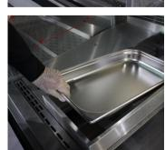
**Step 3**Take out the metal parts, pan frames and/or plates.
