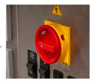
Step 1 IMPORTANT: turn off the Custom Counter main switch by turning the switch as shown.
