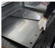
**Step 9**Remove the bottom plate.
