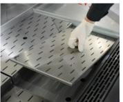
**Step 5**Take out the metal parts, pan frames and/or plates.
