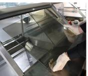
Remove glass sliding doors by pulling it upwards. Then take it out. Be careful that the sliding doors do not get scratched or damaged after removal.
