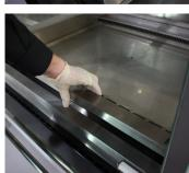
**Step 4**Remove the bottom plate.
