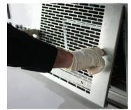
Remove the grid at the front of the condenser by pulling it upwards. Then take it out.
