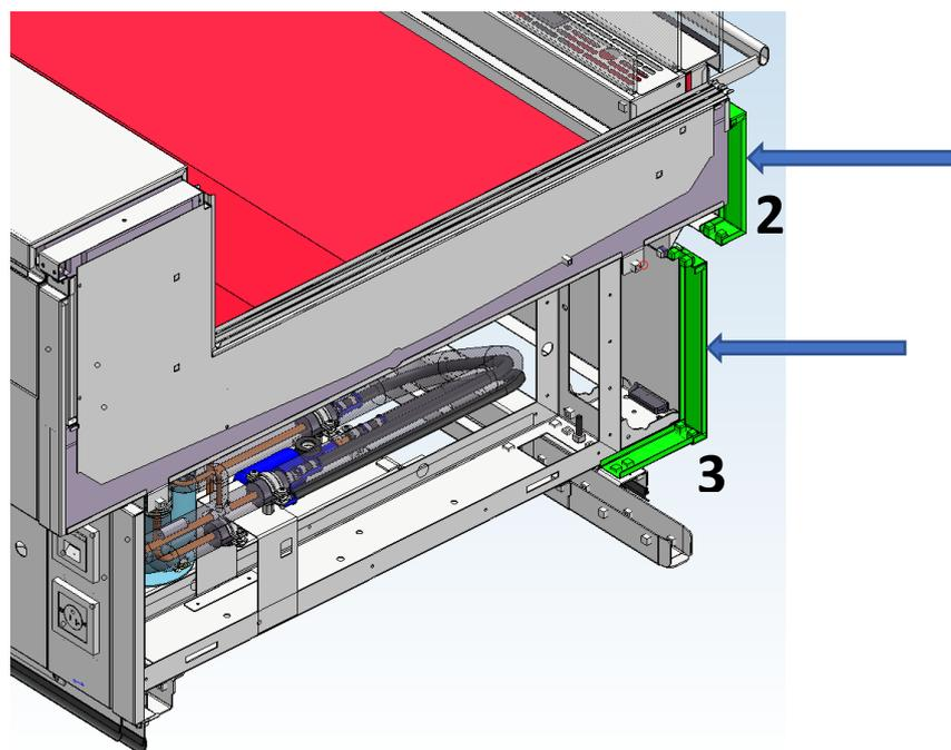
**Step 3.** Remove upper (2) and bottom (3) *front panels* of combination wall
