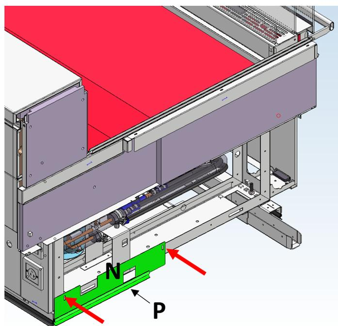
**Step 17.** Mount *plinth (N)* with *sealing (P)*
