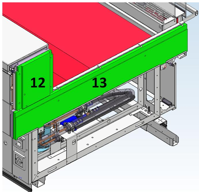
**Step 7.** Remove outer *insulation* parts (12 + 13)
