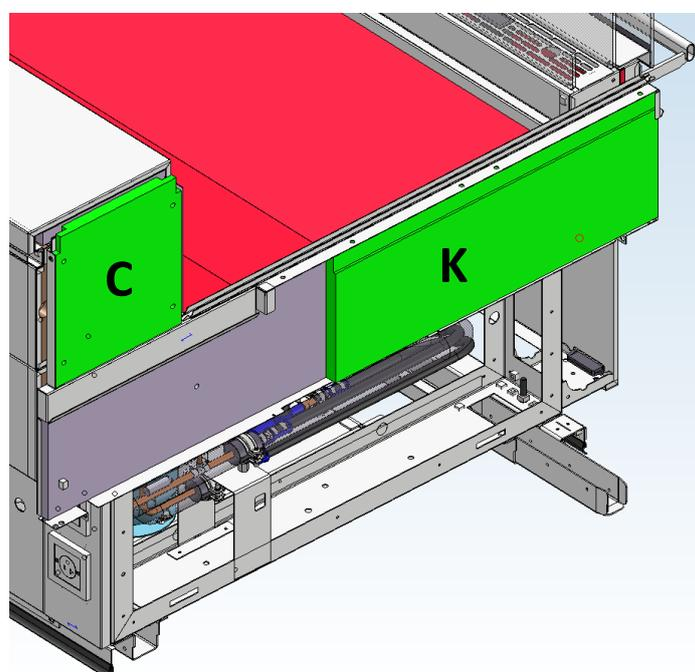
**Step 15.** Place *insulation parts*, of approx. 246 x 265 mm (C) and (K) 630 x 225 mm
