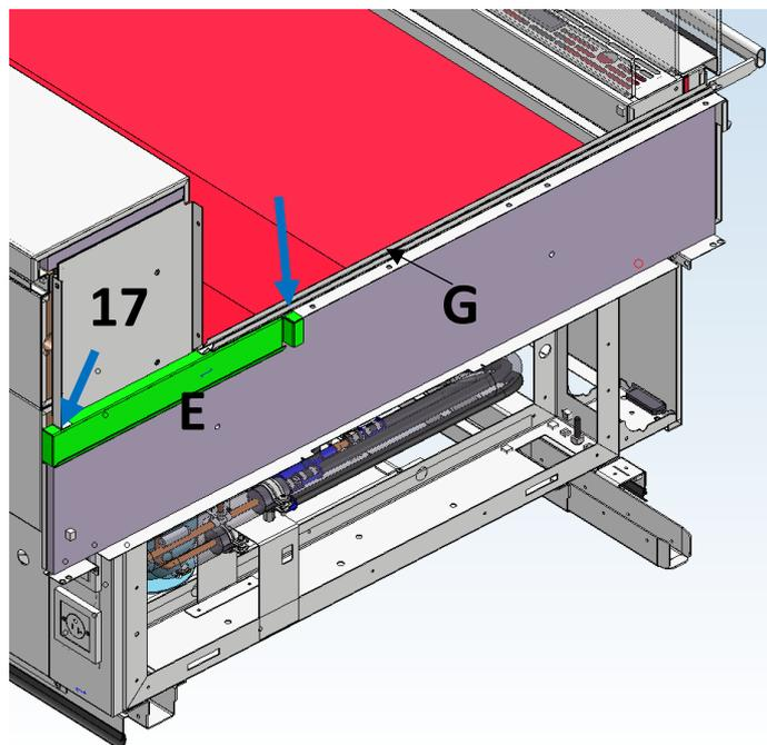
**Step 14.** Mount *base end panel holder (E)* to *L-shaped plate (G)* (mounted in step 12) and *glass holder (17)* (see step 10)
