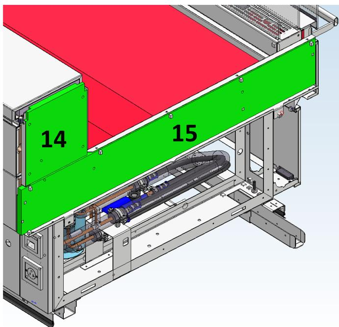
**Step 8.** Remove inner *insulation* parts (14+15)
