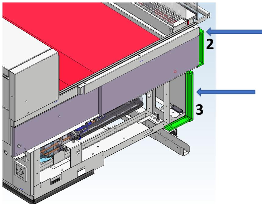
**Step 20.** Mount the *front panels (2+3)* that were removed in “Phase 1 disassembly – step 3”
