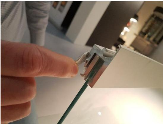
Use a plastic hammer or the back of a screwdriver to put the metal part in place
