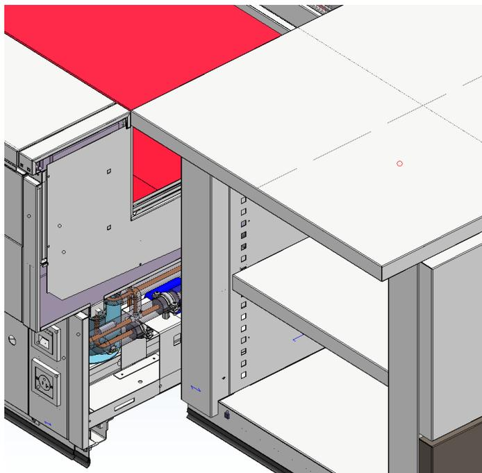
**Step 1.** Move *CC Base* to get free access to side wall and remove end glass of counter
