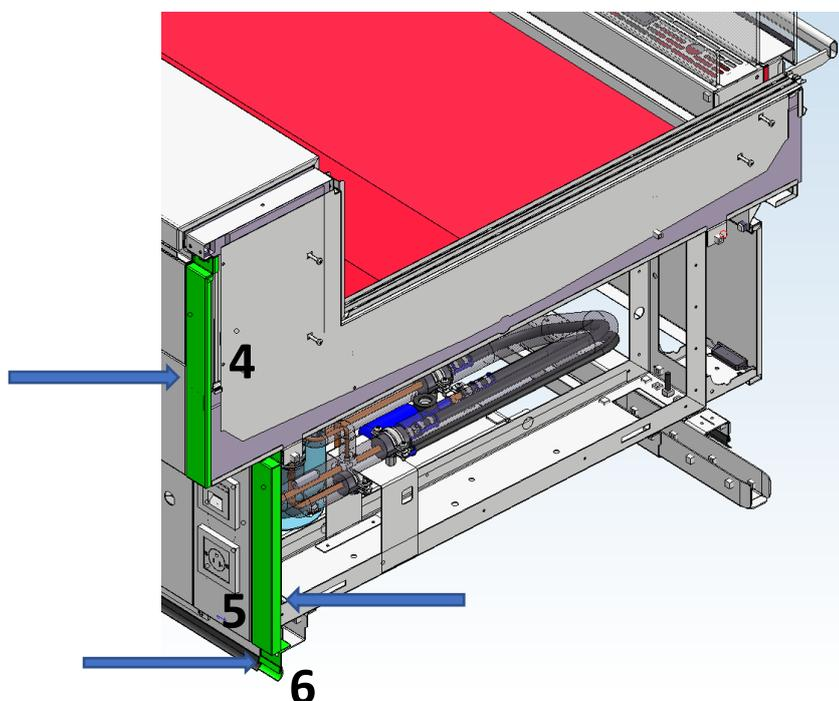
**Step 4.** Remove upper (4) and bottom (5) *rear cover + plinth* (6) of combination wall
