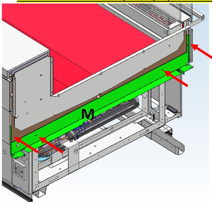
**Step 11.** Mount *mounting profile (M)* to side of counter
