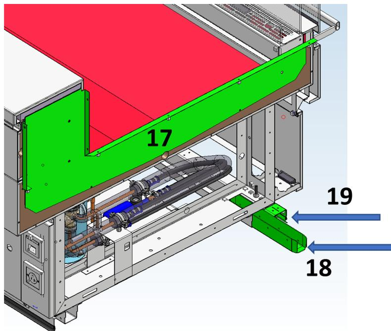
**Step 10.** Starting point: leave L-shaped plate (17), coupling beam (18) and front combination wall plinth (19) on counter
