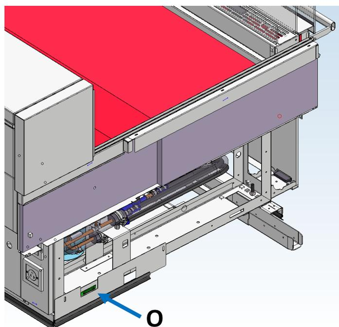
**Step 19.** Place the *magnetic lock (O)* in the opening of the leg
