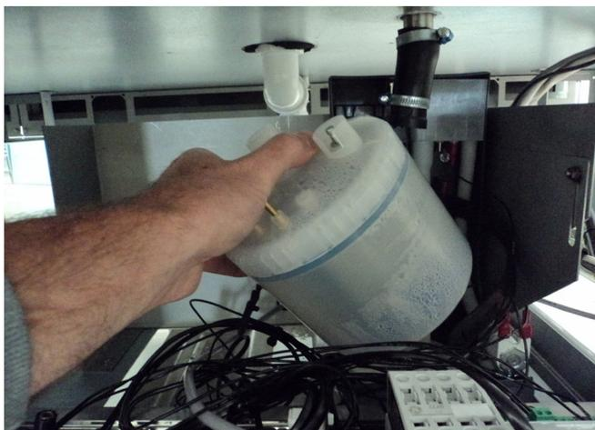
Move the unit upwards and tighten the hose clamp. Tighten the unit with the 3 nuts. Connect all cables, tighten the strap and put the back plate back.
