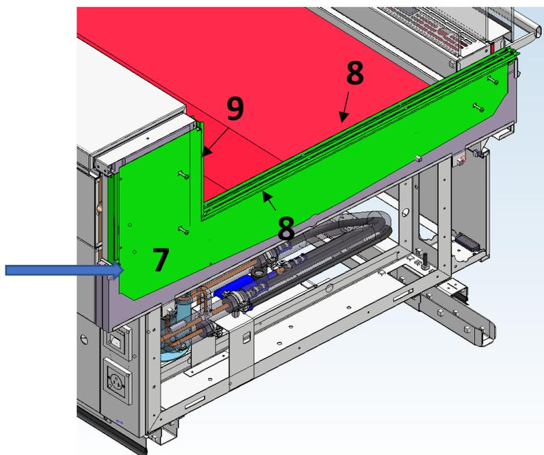
**Step 5.** Remove *L-shaped plate (7)*, *2x horizontal glass holder (8)*, *vertical glass holder (9)*
