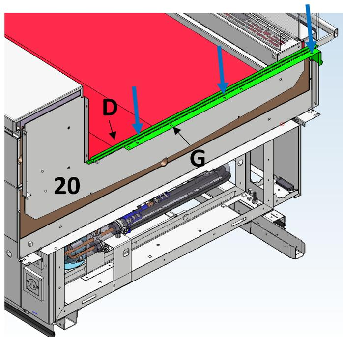
**Step 12.** Mount 2 glass holder parts (D+G) to L-shaped mounting profile 20
