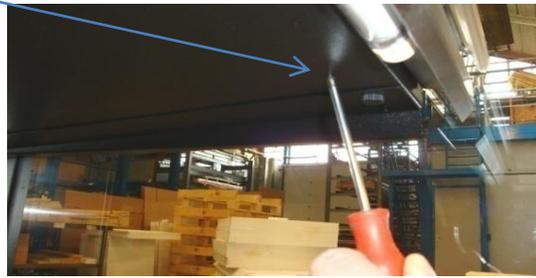
4) secure the temperature indicator with 2 screws. Max. length of screws is 15mm
