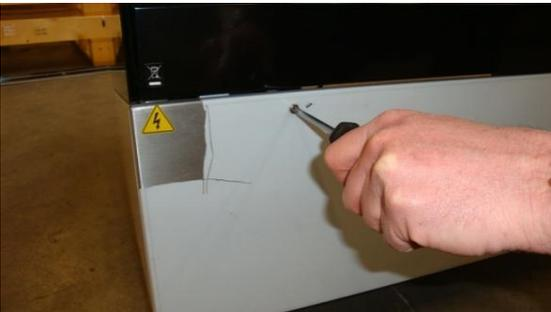
4) Left and right side: (front) remove the screw, and slide the cover plate backwards.
