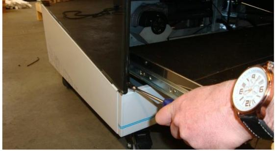
3) Remove the screws left and right on the back side, and remove the cover plate.
