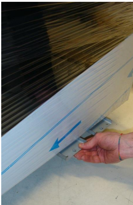
Remove metal brackets 4x
