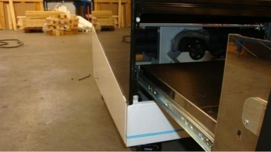
2) Remove the screw on the left and right hand side, and remove the cover plate.
