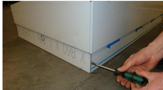
13) Mount the cover plate on the front side and fasten the screws.
