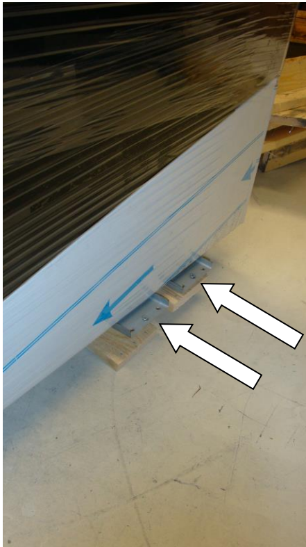
Remove remaining screws
