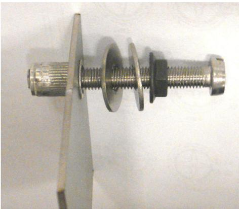
Slam the assembly in the hole with a hammer. (on the bolt head)
