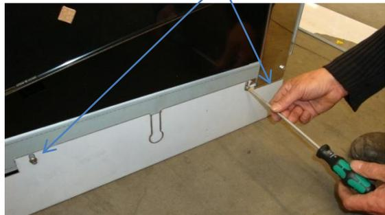
7) Mount both cover plates on the left and right hand side with a screw.
