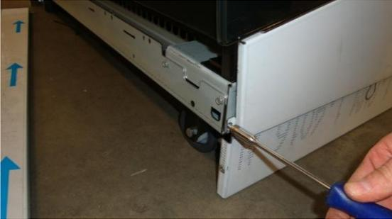
10) Mount back cover plate on the back side inside the slots. Note:
