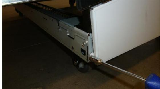
5) Determine where the power cord has to come out of the machine (left, right, back or front) and remove the knock-out of the corresponding lower skirt.
