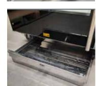
Don't forget to check the fat collector - depending on the TDR model this is, for example, a tray, drawer or bucket.
