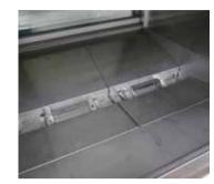
Step 6 Replace filter screens and deflector plates in the correct position, as shown by "checkpoints", see below.
