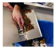
Step 2 Remove the dispenser, deflector plates and filter screens and dispose remains.
