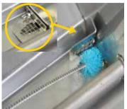
Step 5 Open the filter. Clean the drain under the filter screens with a brush. Push it completely through the drain.
