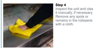
Step 4 Inspect the unit and clean it manually, if necessary. Remove any spots or
