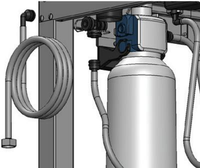
3. Take apart the hoses and the T-fittings on the non-filtered side of the water filter. Use a flat screw driver for the clips.
