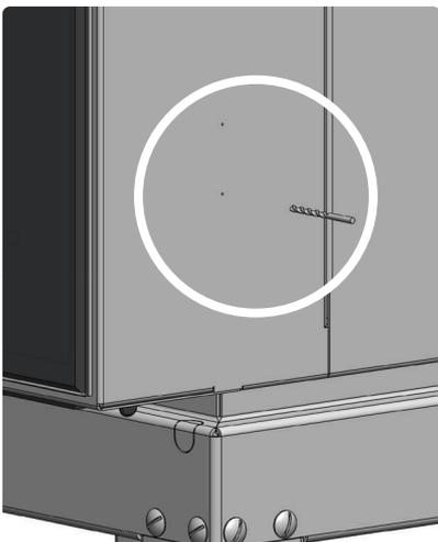
2. Drill two holes at the markings using a 3.3 mm drill.
